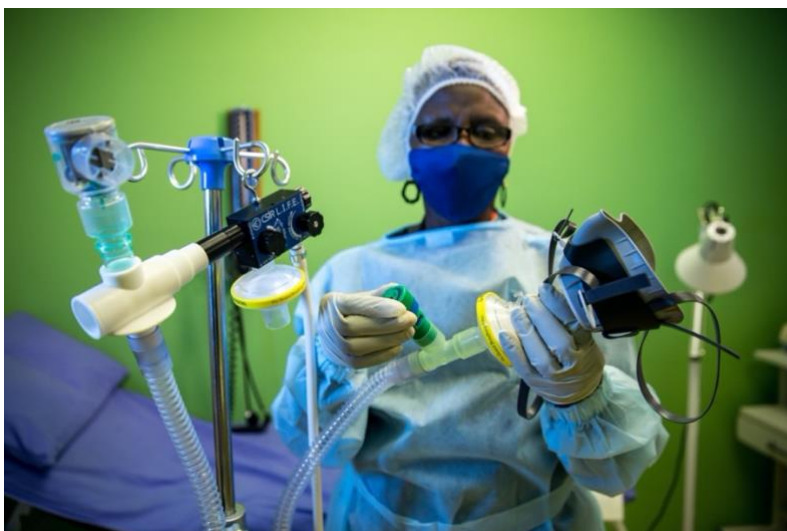
Picture 1: This is a Medical technician holding the entire device, showing the blending unit and patient mask. The device supplies a pressurised mixture of ambient air and industrial oxygen to the patient through a mask or hood.
