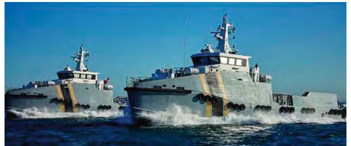
35m Sentinel crew & patrol vessels by Nautic: 28 knots, ballistic protected, fly-by-wire. 30 days of mission time between resupplies.
