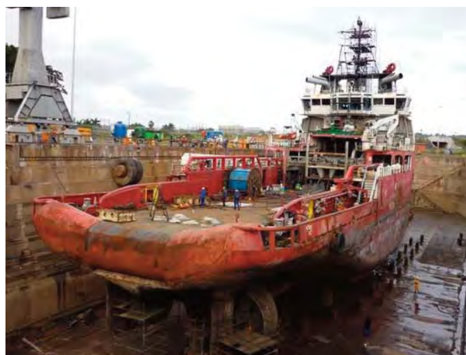
Electrical refit and full powertrain overhaul of the fire-damaged offshore tug Subhiksha, by Southern African Shipyards. A complete overhaul to the main engine and crankshaft; thrusters, propellers and main shaft. Replacement of all electrical items, including over 15km of wiring.
