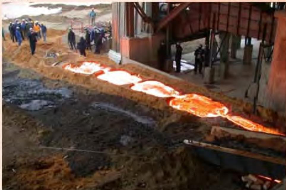
Chrome running out of furnace into forms
