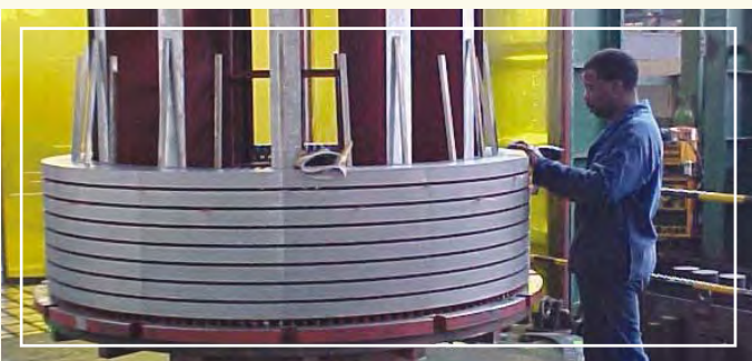
Operator assembling components forming part of a large electrical motor at the ALSTOM factory in Benoni
