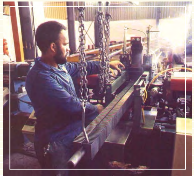
Welding of H fins onto an economizer tubing, as part of a large watertube boiler contract, at the group's John Thompson factory in Bellville, Western Cape
