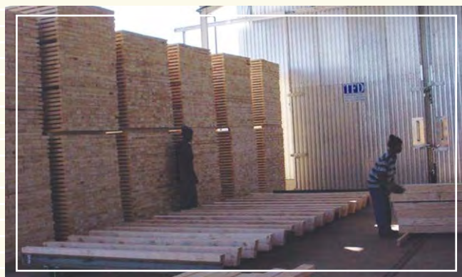
Wood to be treated in the new kiln
