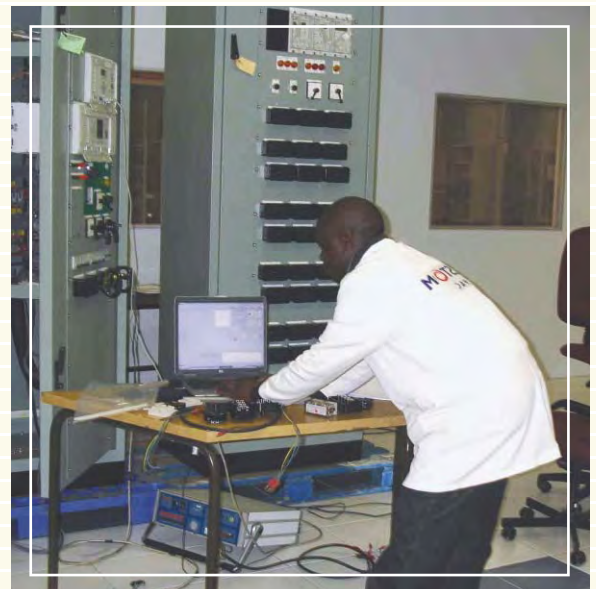
A Test Technician busy programming a Current Differential Protection Scheme for export to Sudan in the Test Bay at the ALSTOM Protection & Control site in Knights, Boksburg.
