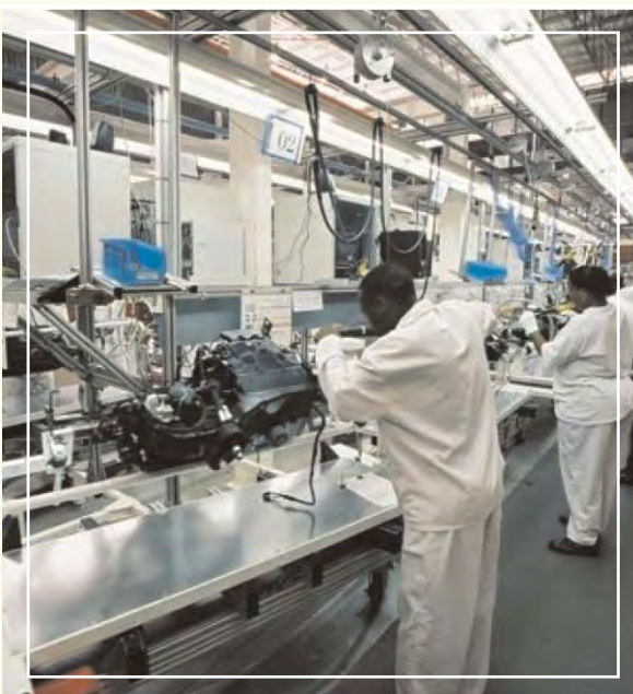
Initial stages of the cockpit assembly line
