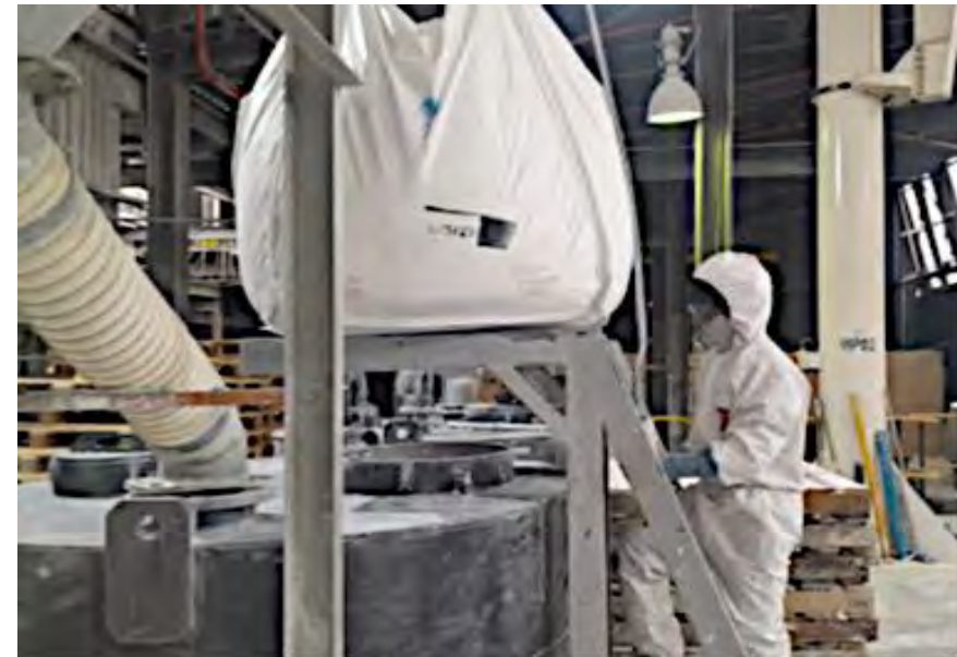
Titanium pigment bulk bags being loaded into hoppers and mastermix high speed dispersers and stored
