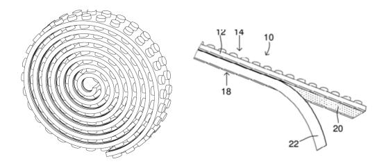
The base is flexible, cuttable with scissors, and includes an adhesive (20) with a removable cover (22) on one side so that you can stick down the base and build Lego structures in various ways. The base is long (up to 1m) and packaged in a roll.
