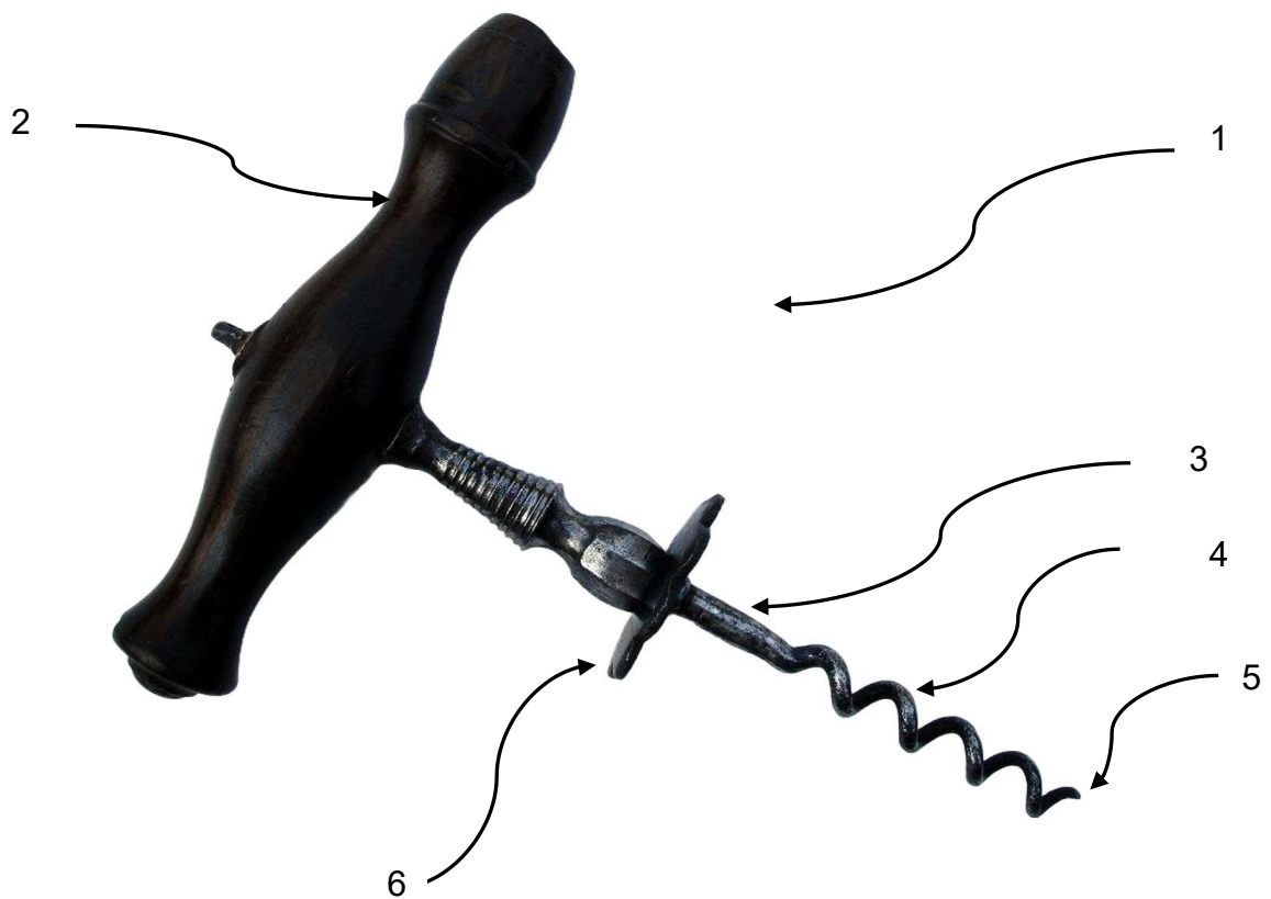
Figure 2 (Prior Art 2 – Basic Corkscrew with Henshall Button)
