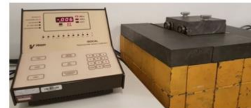
Photo 1: The calibrated NMISA secondary standard ionization chamber which was used to perform calibrations of various radionuclides for NTP Radioisotopes and nuclear medicine facilities.
