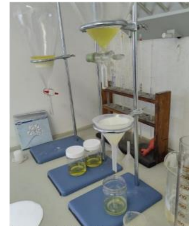
Photo 2: Liquid-liquid extraction process of the samples
