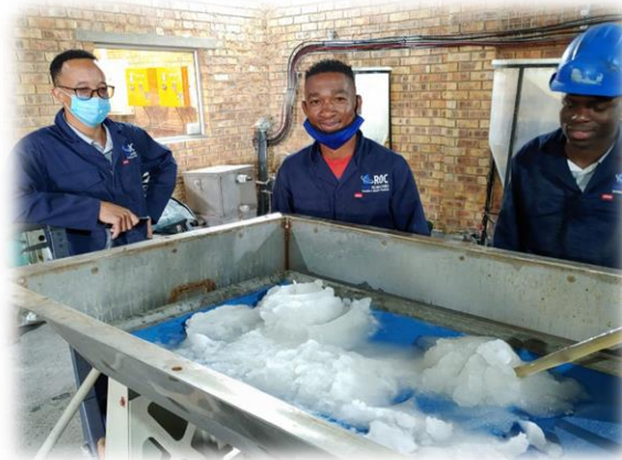
Students looking after Freeze crystallisation. Recovery of \text{Na}_2\text{SO}_4 through cooling.
