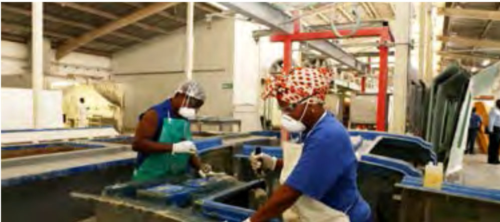
Moulding stage of Bell E-Series hoods
