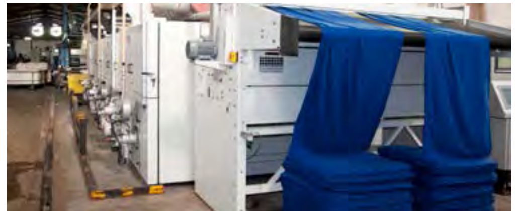
The new Bruckner tubular dryer installed at Dyefin
