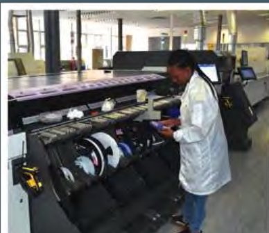
Components are loaded on reels that feed into the Pick and Place machines
