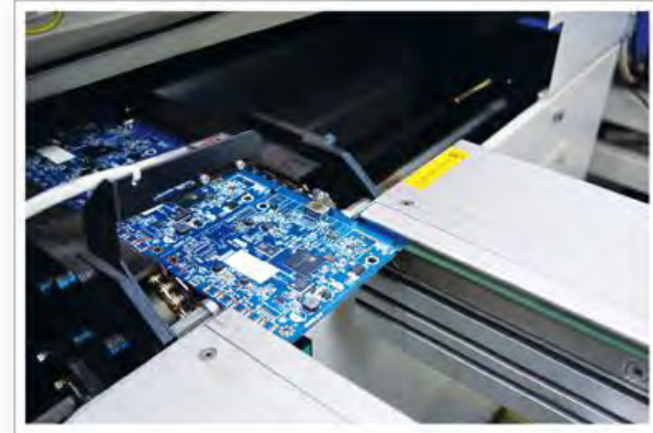
Pick and Place machines add on components to the board while it goes through the production line
