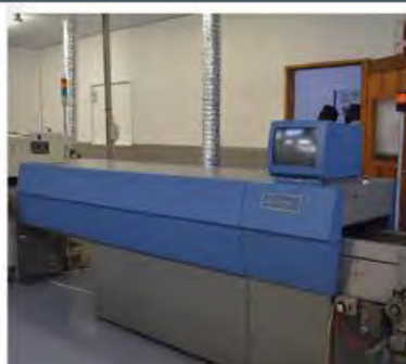
The Conformal Coater provides a protective layer over the boards
